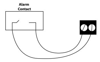
The Wireless Dry Contact sensor will, by default, be set to accept a Normally Open contact. To change the input type to a Normally Closed contact, you can use the web page or use the keypad on the WSG30. To use the keypad, press the Menu button, then select Inputs. Scroll to the dry contact sensor you wish to change and press Enter. Next, scroll down to the Type and press Enter. Choose either N.O. or N.C. and press Save.
