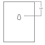
Use a pencil to mark the hole locations at the top and bottom of the housing. Install the drywall anchors (if necessary) to the wall. Attach the housing to the wall using #6 tapping screws.
