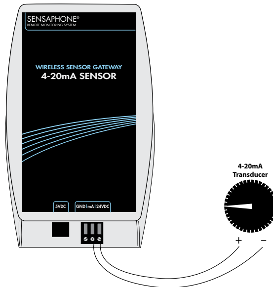
4-20mA Transducer using 24VDC power supply
